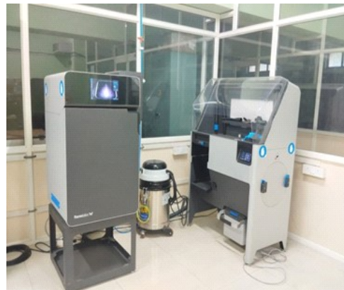
3D printer Selective laser sintering (SLS) Formlabs Model : Fuse 1+30w
