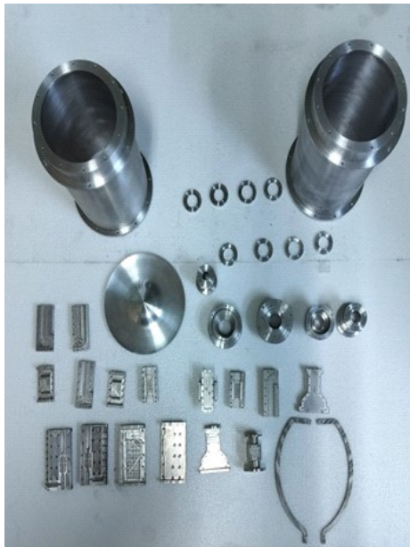
Feed Components of Satellite Communication
