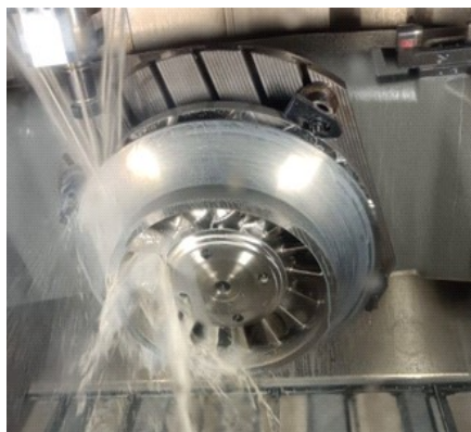
Closed Impeller job on 5-Axis Hurmule-650C, CNC Machine
