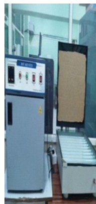
Solder masking and legend printing setup stand
